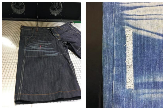
Fig.3 Laser engraved cat whiskers on jeans and hole-punching effect
